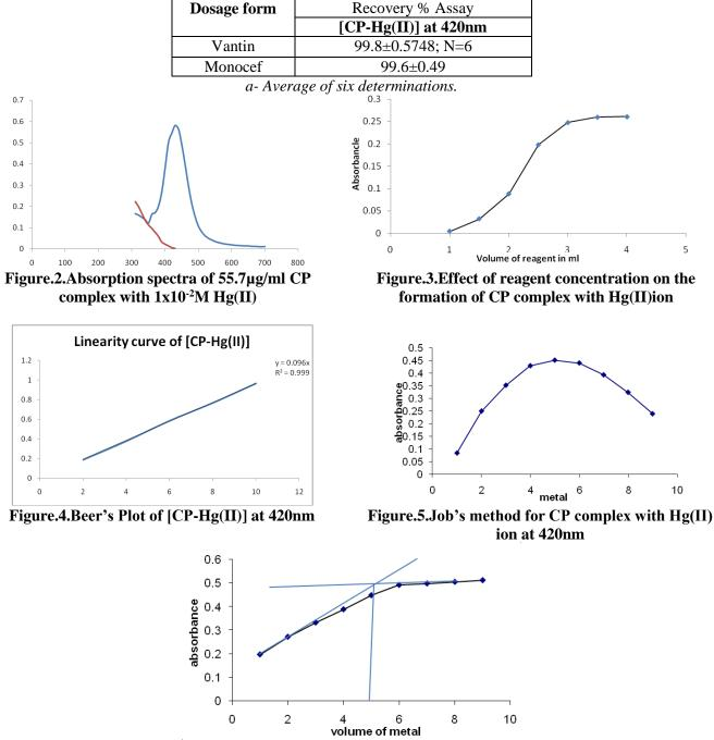
Figure.6.Mole ratio method for CP complex with Hg(II) ion at 420nm
